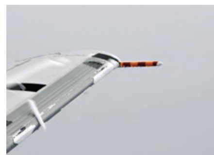
Icing test: the moment when the wing boot broke the ice.
