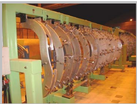
Phenom 300 central fuselage assembly jig
